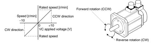
The following table indicates the rotation direction according to forward rotation start (ST1) and reverse rotation start (ST2) combination:
